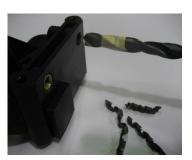
Using a variable speed drill, slowly drill out the existing hole to the needed depth. It is important to drill the hole directly in-line with the existing hole. Any out of squareness may reduce the success of this installation. It is also important to not oversize the drilled hole. This will reduce the holding power of the insert.
