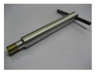
Thread insert onto installation tool as shown:
