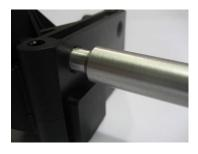
Stop once the insert is to desired depth. It should be slightly below the surface of the part. On parts with an angled parting line, such as the front gearbox halves of the Losi 5ive, the insert will have to be installed deeper to allow the two halves to seat on each other.
