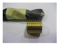
Determine the depth of hole needed and mark the bit with a marker or tape as shown here. The depth of the hole needs to be deep enough so the insert can be installed flush or below the surface of the part.
