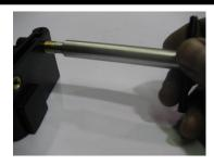
Screw insert into part as shown. Be careful to hold it perpendicular in both directions as you install the insert.
