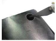
Chamfer the hole slightly with a hobby knife or similar. This will help the insert start cleanly.
