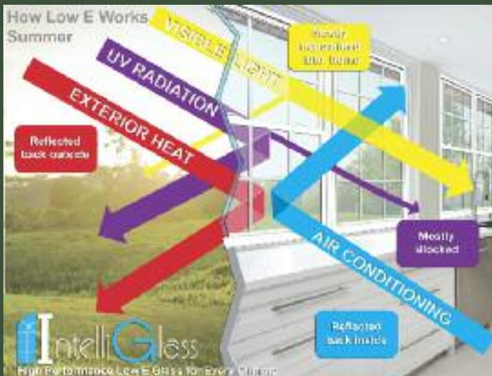
In predominantly **cooling** environments, IntelliGlass reflects exterior heat away from your home. Solar radiation is filtered to preserve the comfortable indoor temperature the air conditioner provides. Most UV radiation is blocked, while a high amount of visible light shines through.
