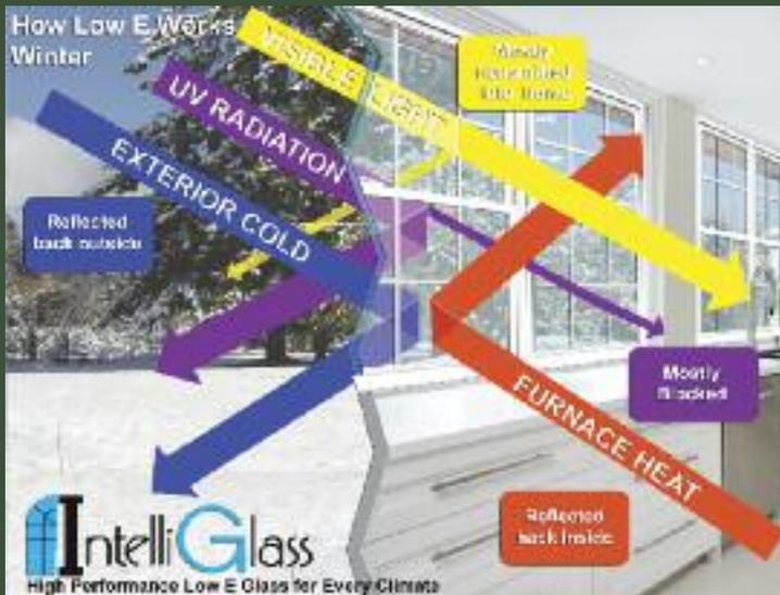
In predominantly **heating** environments, IntelliGlass reflects furnace heat back into the home, reducing the burden on the furnace, yet keeping your home warm and comfortable. Some solar radiation passes through the glass, acting as a source of free energy. Most UV radiation is blocked, while a high amount of visible light shines through.
