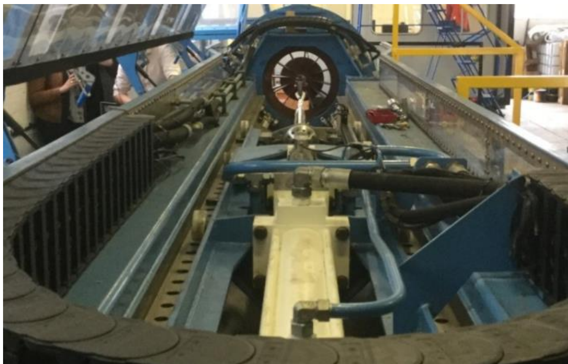
FIGURE 3 - DMAC TEST RIG - SHOWING THE SET-UP OF A DESTRUCTIVE TENSILE STRENGTH OF A SYNTHETIC MOORING LINE
