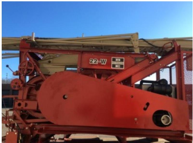
Completely refurbished 22-W with new Perkins engine and levelling jacks for easier setup.
