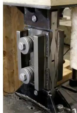
As shown, the RSFJ hold-downs were installed in the notches at the bottom corners of the CLT wall. The RSFJ configuration was composed of two centre slotted plates and two cap plates.
