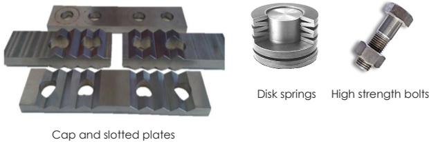
The outer cap plates and the centre slotted plates are grooved and clamped together with high strength bolts and disc springs. When the applied joint force overcomes the frictional resistance between the sloped bearing surfaces, the centre slotted plates start to slide and energy will be dissipated through friction during cycles of sliding.
