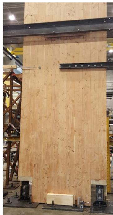
Large-scale shear wall testing using RSFJ as hold-downs
