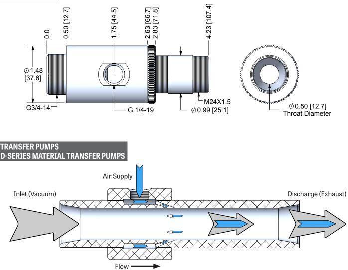
Direct Transfer Pumps use high velocity compressed air to generate a vacuum in the inlet of a smooth bore tubular body to drawn in bulk dry goods and then convey it in a turbulent air stream through a hose attached to the discharge end of the pump. Plastic pellets, powders, beans, peas, sawdust, and continuous fabric trimmings are only a few examples of the numerous items that can be transferred.
