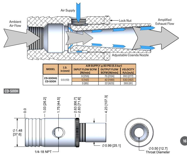
All performance data presented is a representatation of production pumps but is not a guarantee due to variations in local barometric pressure and of mass produced components.
