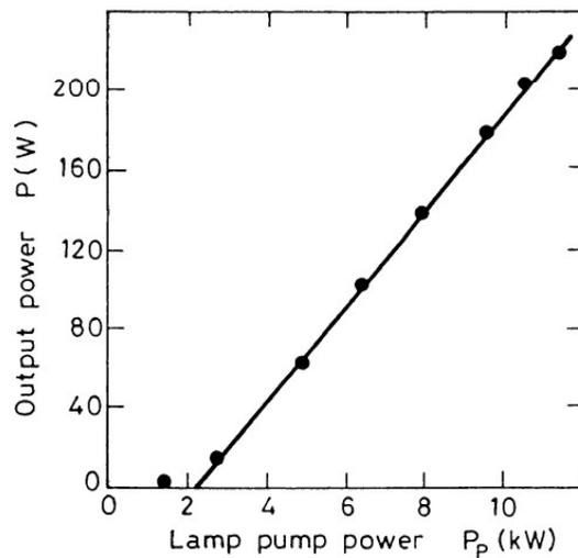
FIG. 7.5. Output power vs lamp input power for a powerful Nd:YAG laser (after Koechner,<sup>(7)</sup> by permission).
