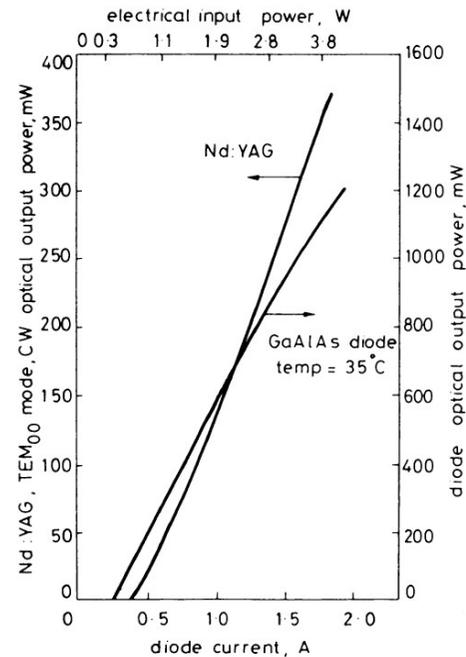
FIG. 7.13. Output power vs diode current for the Nd:YAG laser of Fig. 7.12. In the same figure the output power vs current of the laser diode array is also shown (after ref.,<sup>(15)</sup> by permission).
