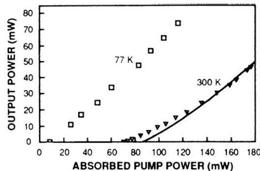
FIG. 7.14. Plots of the output power vs absorbed pump power for a Ti:sapphire-pumped Yb:YAG laser, for liquid nitrogen cooled operation (77 K) and at room temperature operation (300 K) (after ref.,<sup>(18)</sup> by permission).
