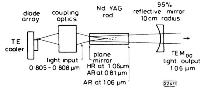
FIG. 7.12. Schematic illustration of the experimental set-up of a Nd:YAG laser, longitudinally pumped by a diode array (after ref.,<sup>(15)</sup> by permission).
