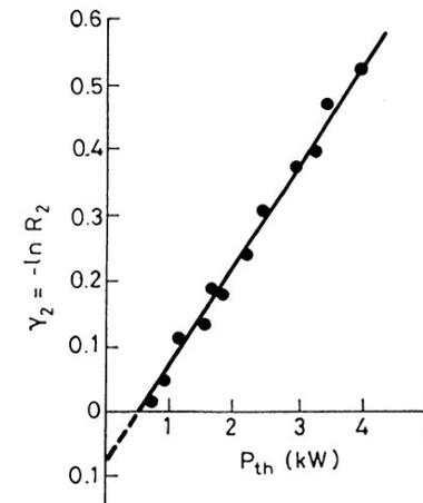
FIG. 7.6. Threshold pump power as a function of mirror reflectivity (after Koechner,<sup>(8)</sup> by permission).
