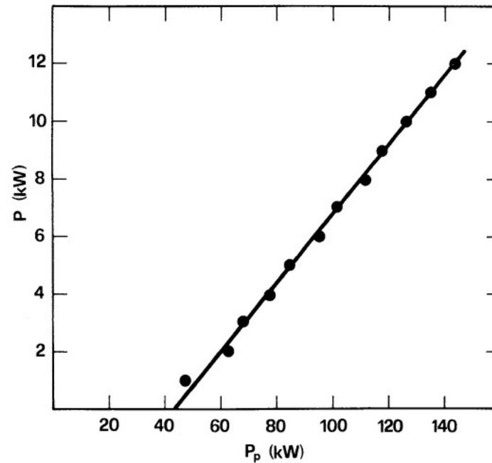
FIG. 7.8. Output power,  $P$ , versus electrical discharge power,  $P_p$ , for a powerful cw CO<sub>2</sub> laser.
