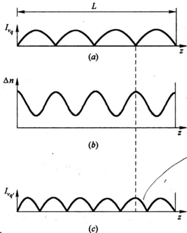
□ This is **because the standing wave effect**. For a certain mode, the field intensity is largest at the antinode while smallest at the node. Correspondingly, the population inversion/gain is the smallest at the antinode while largest at the node. This phenomenon is called **spatial hole burning of the gain**.
