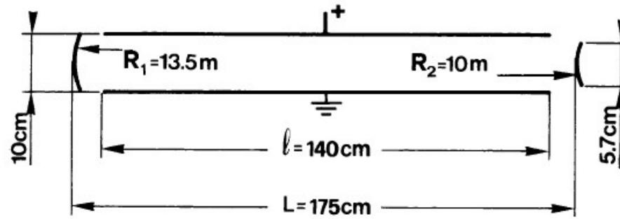
FIG. 7.7. Possible cavity configuration for a powerful cw CO<sub>2</sub> laser.
