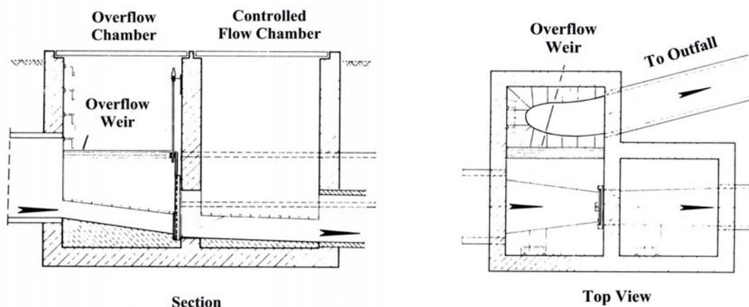
Figure 2: *HYDROVEX® FluidGate control valve implemented in a double chamber (overflow + drainage)*
