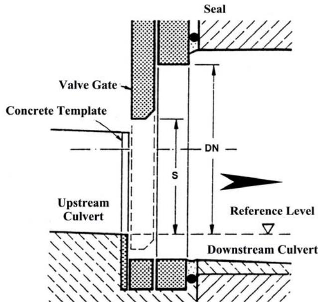
*Figure 3: Section through installed HYDROVEX® FluidGate control valve. When closing, the gate takes over the entire closing section, no « pocket » being created.*
