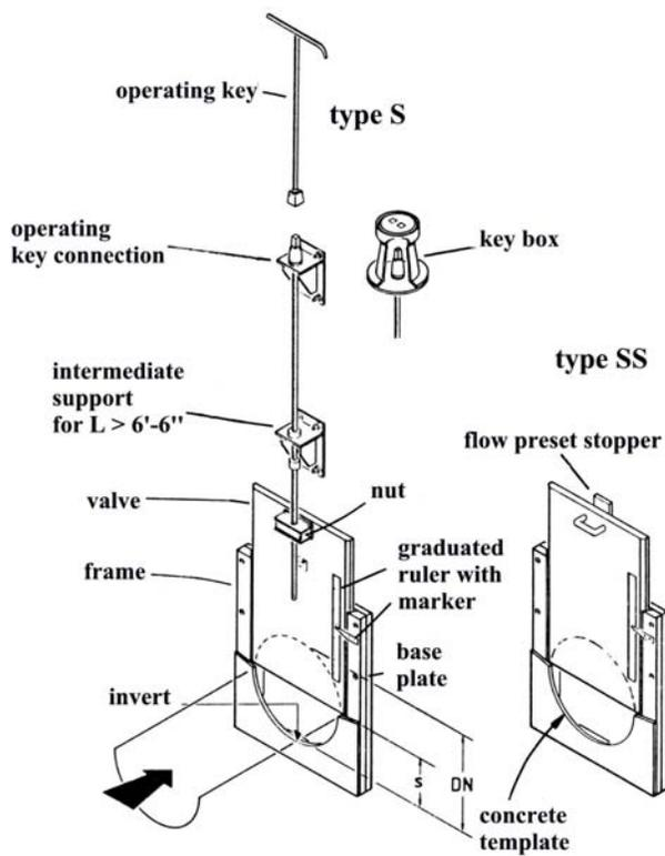
Figure 1: *HYDROVEX® FluidGate control valve with extended threaded rod for sufficiently deep chambers type « S », or chambers that are shallow with wedge adjustment, corner type « SS ».*
