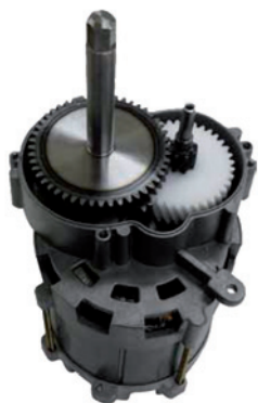
Powerful reducing condensing induction motor slowed to 47 Rpm for gentle squeezing and optimum juice extraction
