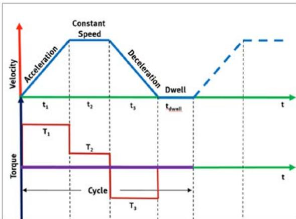
The servo motor's main feature is the capability to develop peak torque for 1-3 seconds, so for an indexing application the entire move is usually only acceleration/deceleration, with acceleration using the peak torque of the motor.
