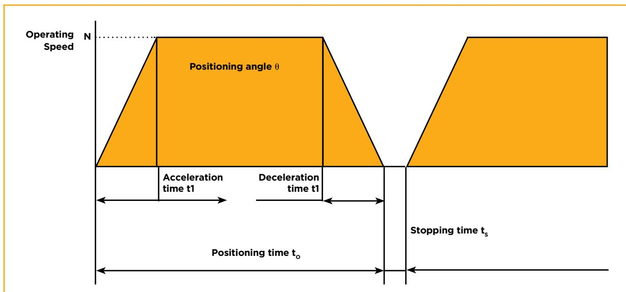
Last, calculate for the required torque,  $T$ , in lb-in. The required torque is made up of the combination of the acceleration torque,  $T_a$ , and the load torque,  $T_L$ . First calculate the acceleration torque,  $T_a$ .  $T_a = ((1.2J_L) / 386)(V_m / (9.55t_i))(1/16)$ , where  $J_L$  is the total system inertia,  $V_m$  is speed of the motor, and  $t_i$  is the acceleration /deceleration time.
