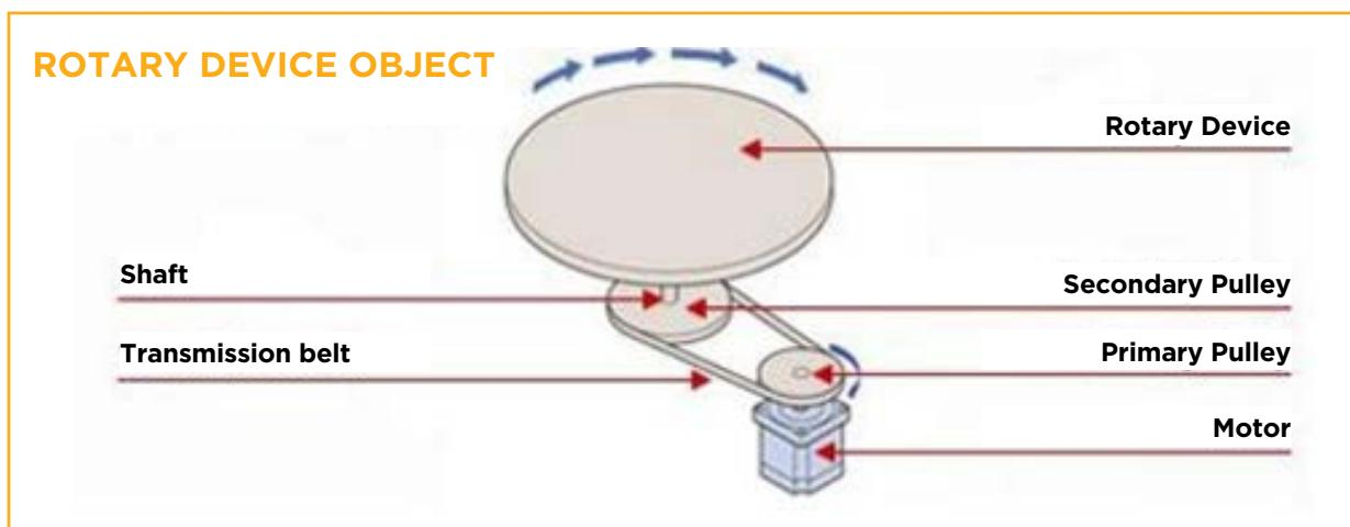
also need to be calculated. To calculate the inertia of the drive shaft use the following equation:  $J_s = (1/8) m_2 D_2^2$ , where  $m_2$  is the weight of the shaft in ounces and  $D_2$  is the diameter of the shaft in inches.
