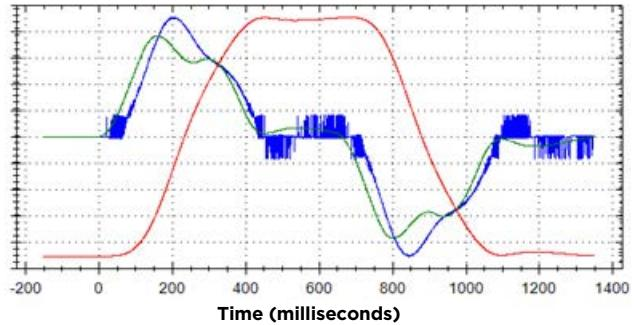
Because the higher resolution feedback is providing twice as much information, 8196/rev, corrections are made much sooner and require less adjustment. In diagram we can see the peaks for the velocity feedback are much lower.
