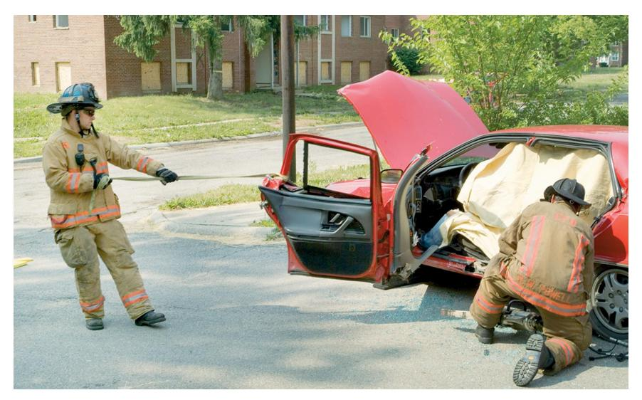
Hydraulic cutters are used to cut the roof from a vehicle.
