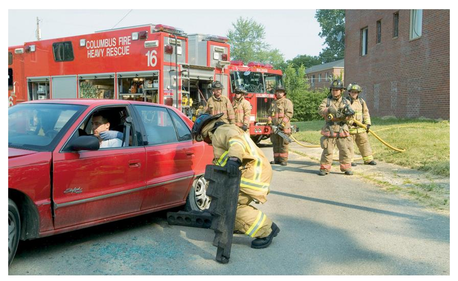
The first step in stabilizing the vehicle is to place chocks under the vehicle. Chocks should be pushed in until they touch the undercarriage; the vehicle should not be lifted up to fit the chocks into place.
