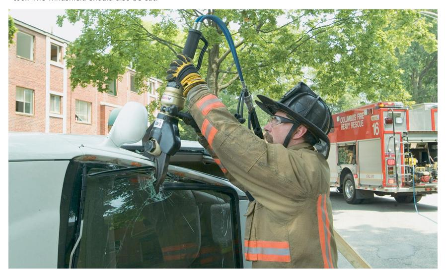
Then fold the roof down to provide an adequate space from which to remove the patient.
