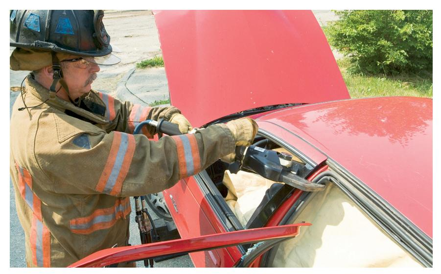
Cut the B post at the bottom by the floor.
