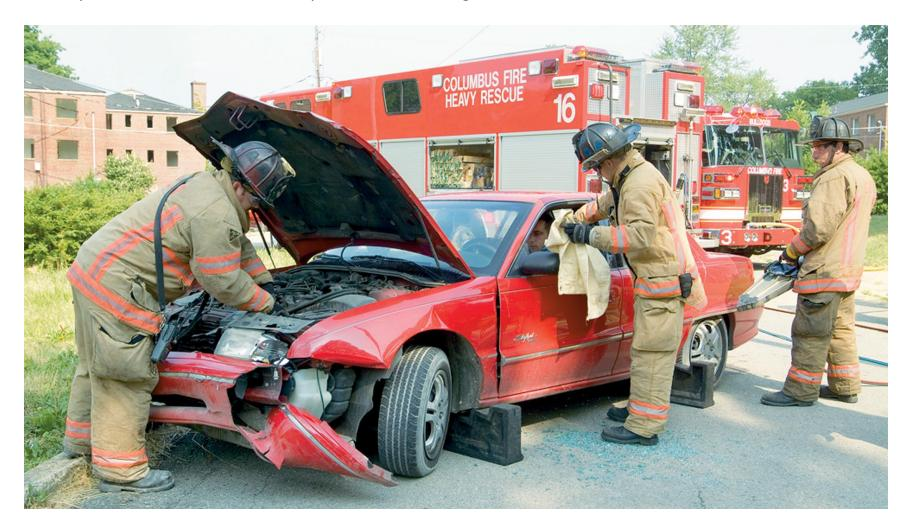
Hydraulic spreaders are used to "pop" open the rear door.
