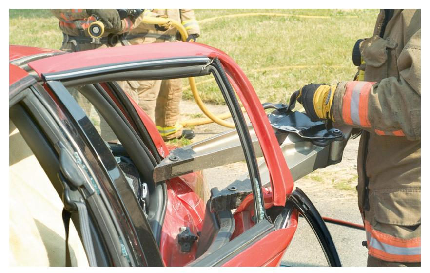
Cut the B post at the top by the roof.
