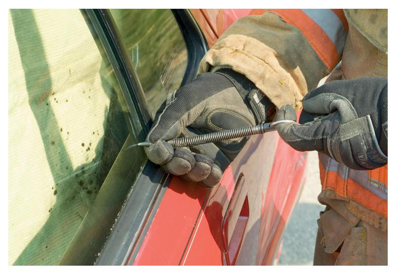
Keeping the tip of the punch in place, let go of the spring to shatter the window.
