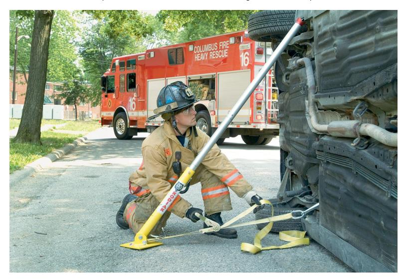
For extra safety, rescue struts can be placed against both the underside and the top of a vehicle on its side.
