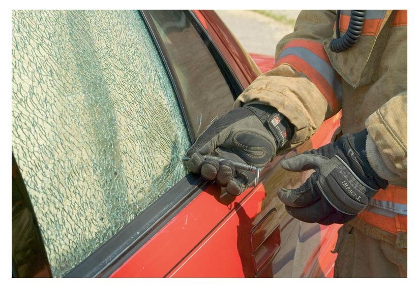
Starting at the top of the window, carefully push the broken glass away from the interior of the vehicle.
