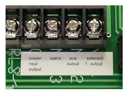
The Outputs for both the Solenoid and the Aux should never have any outside power source applied to them **Severe Damage** to the controller could result!! GSI will not be liable of repair or replacement needed out of any damage of this type.
