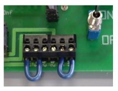
Seen here for 110vac, the 110vac that powers the Roller-Up controller will be used for the external outputs. This circuit should not exceed 4 amps total. For the long life of the controller it is better to activate a relay for external lighting if the aux is used in this manner. Solenoids for a Prep/soap arch should not need an interfacing relay. However a fuse should be used on it so it can not exceed 4 amps.
