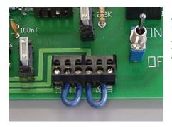
Seen here for 24vac, the power is set to come from the on board transformer. It can drive up to 1 amp of power for the external outputs. This is plenty for an air solenoid and a control relay.
