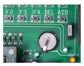
The battery is located just under the 'DEL' key on the circuit board. It is used to back up the user settings. Under normal operation the battery should be replaced every 5 years. Once the battery goes out the user data would be lost upon the loss of power. When this kind of loss happens, the user settings may get garbled and the values corrupted. If this ever happens due to battery change or a main board exchange it is easy to reset to factory settings and reprogram.
