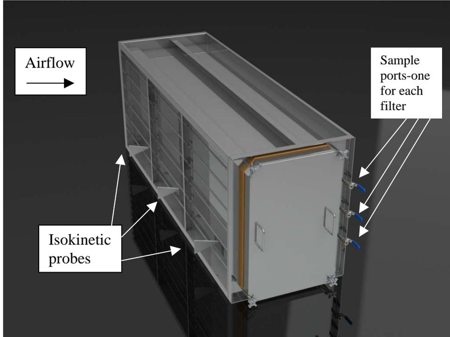
P&G Mfg (Model No. SIH-10H30W-304) 1 x 3 scan housing shown with door attached
