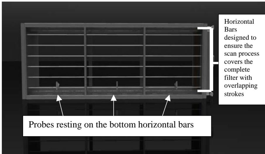
P&G Mfg (Model No. SIH-10H30W-304) 1 x 3 scan housing shown in upstream view
