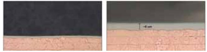
**FIGURE 4.** Cross section showing plated Cu with bright Ni smoothing layer to decrease surface scattering.
