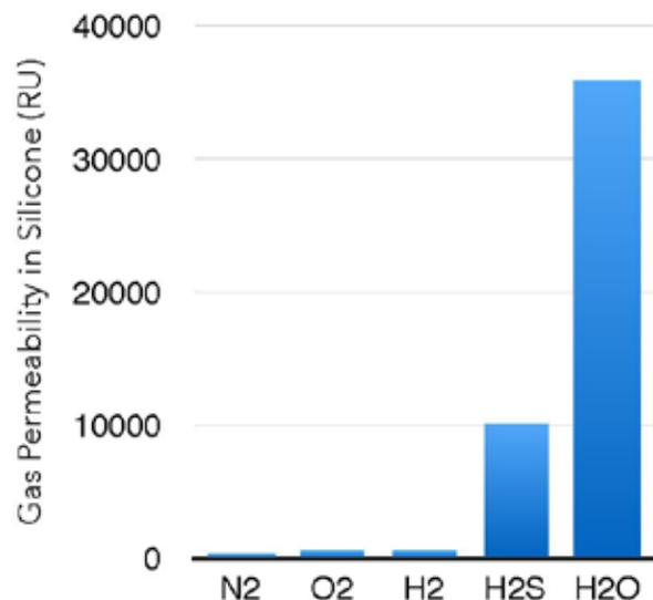
**FIGURE 2.** Gas permeation rates through silicone (relative).
