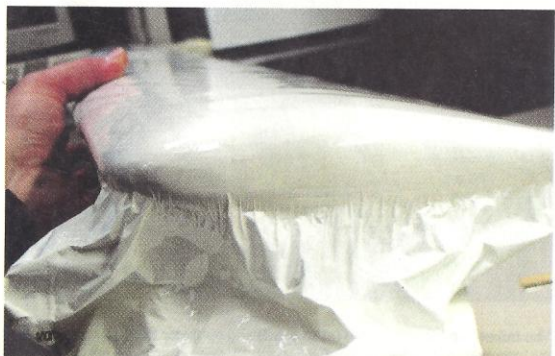
lage. Fillets (below left) were used to soften the lines of the wing to flap to fuselage joint. The Hangar 9 Ultracote (below right) can readily stretch around curved sections of the wing tip. Practice with different settings on your iron, as the dial heat indicators are often not similar on various brands of irons.
