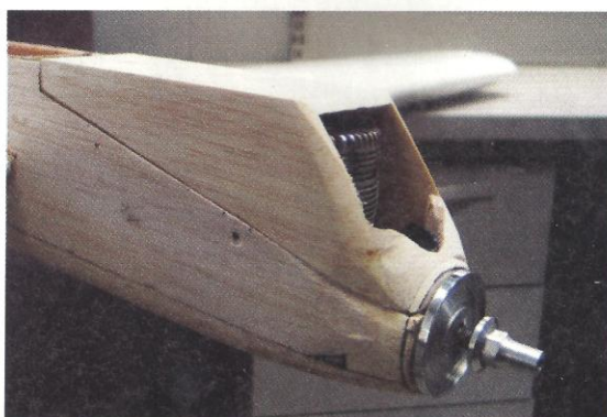
Michael's prototype of the Encore 50, a PA .61 was installed (above right) on the engine crutch. At this point the cowl blocks are merely roughed out.
