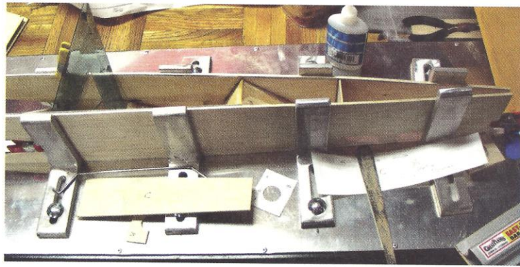
The rear fuselage is held steady in Byron Barker's (C.F. Slattery) fuselage jig. He can be reached at either 812-944-8511 or 812-948-9167 to purchase this precision tool.
