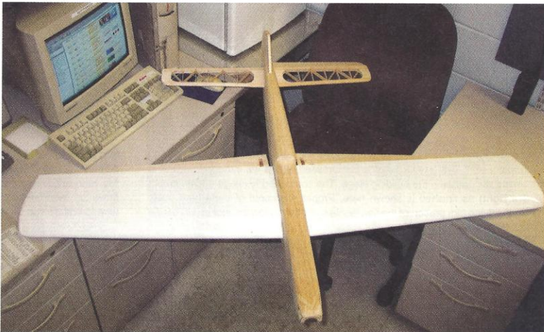
The Encore begins to take its final shape. Instead of the classic dope finish, Michael chose to use Ultracote, and at this point has covered the wing with it after installing leadouts and bellcrank first.
