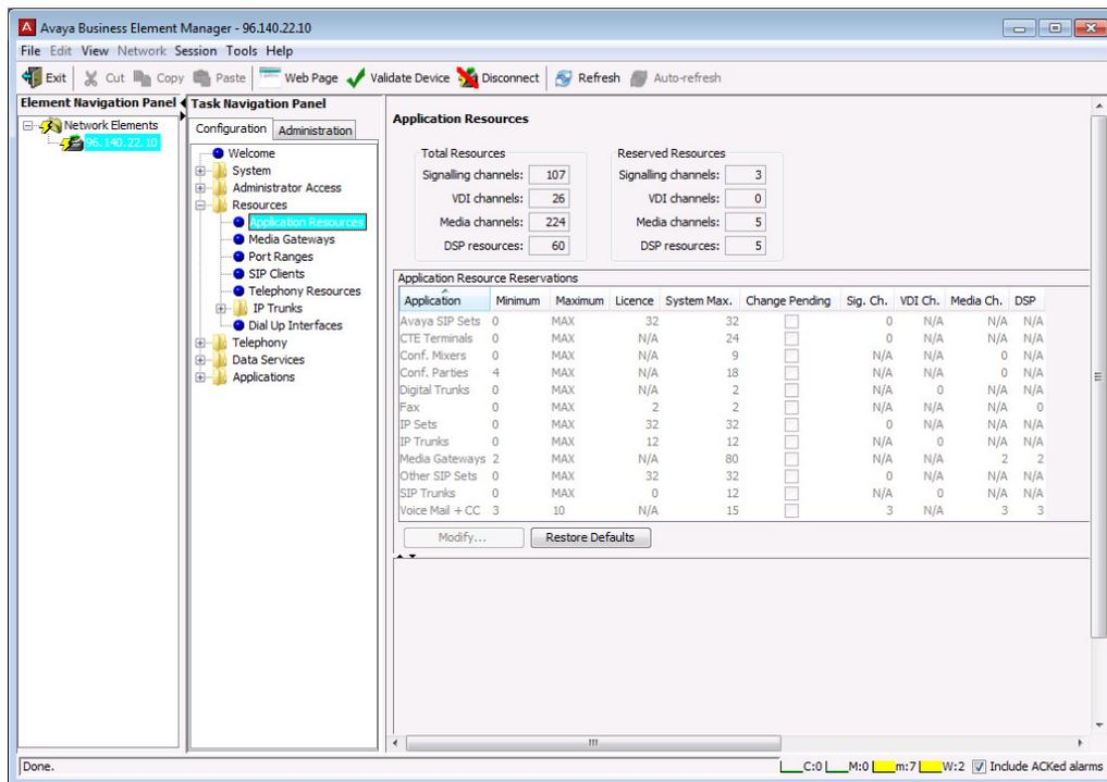
The Nortel SIP Sets line was replaced with Avaya SIP Sets. A new “SIP Client” area appears at 6.0.
