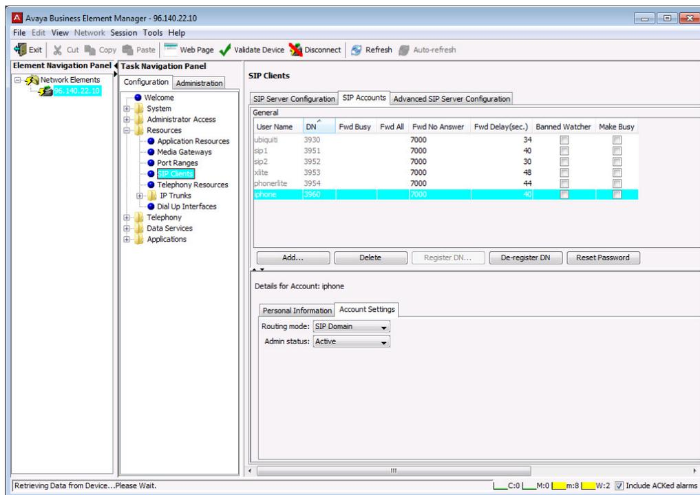
Click on the "Add" tab and enter in the name (which must match the name entered on the SIP device!) without any spaces. Add in the DN or tick the Auto assign box. Click OK to add it in.
