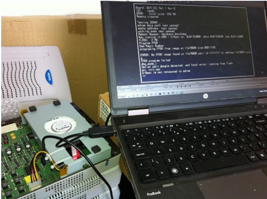
The serial port connector on a BCM 50b is located below the BRI module and you will probably need to remove the board after powering off the BCM first to insert the serial cable and then replace the module, before powering it up again as shown below with the BRI module attached. Be aware that the **bridging pins are on the right** towards the hard disk power connector.
