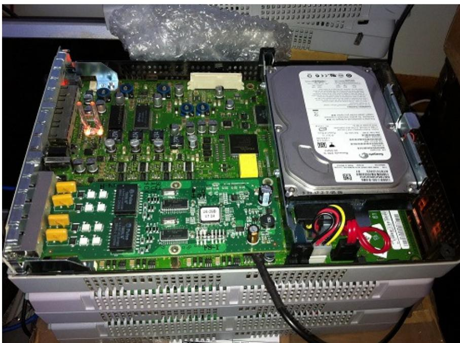
A close up of the serial cable and coloured wires is shown here attached onto a standard BCM 50. Please be aware that only three wires are needed and the Red 3.3 volts lead isn't used!. Also a green IDE jumper was used to bridge the pins needed for the u-boot console to work.
