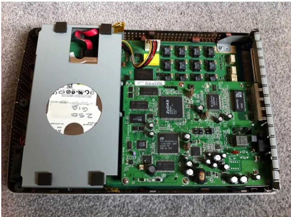
The BCM 50 "b" has a different (Type 2) Motherboard and it uses a connector that exists near to the top because the board that sits over the serial port pins has two BRI ports that go over the 25 pair Viking connector. An example of a BCM 50b is shown below
