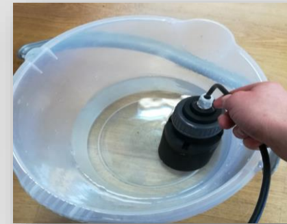
Place the Dip Probe into distilled water
