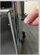
1. Connect handle to the back of the machine using the 4 wing nuts provided.
