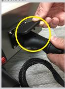
**6.** Lift the flap and connect the hose ensuring the pin locks into position.
