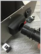
5. Connect vacuum hose, clicking it into position. Ensure it cannot be pulled out.
