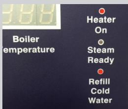
15. Refill Cold water when the refill cold water light illuminates and a intermittent beeping noise can also be heard.
