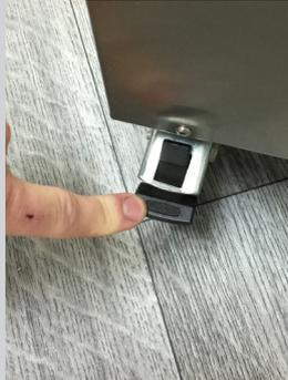
7. Push your machine to a suitable area and lock the brake lever to avoid the machine moving during use.
