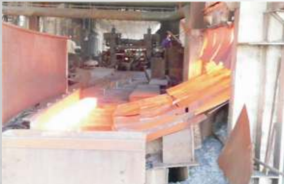
Vyberanie ingotov s antioxidantom po nahriatí Removing ingots with antioxidant after warming
