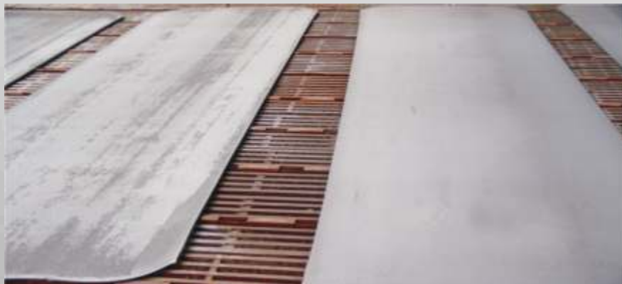
Porovnanie oxidácie na povrchu oceli ( vľavo bez a vpravo s antioxidantom ) Comparison of oxidation on the surface of steel (left and right with no antioxidant)
