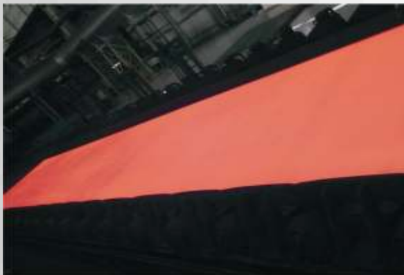
Bežná oceľ s antioxidantom po nahriatí Ordinary steel with antioxidant after warming
