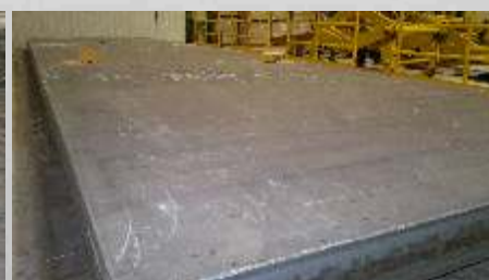
Povrch po valcovaní s antioxidantom Surface after rolling with antioxidant
