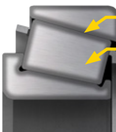
Cross-sectional view of a bearing made from case-hardened steel
