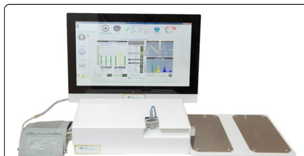
Figure 1 Photograph of the TM-Oxi and SudoPath system. This machine is a software complex managing three FDA cleared devices; a blood pressure device, an oximeter, and a galvanic skin response device.
