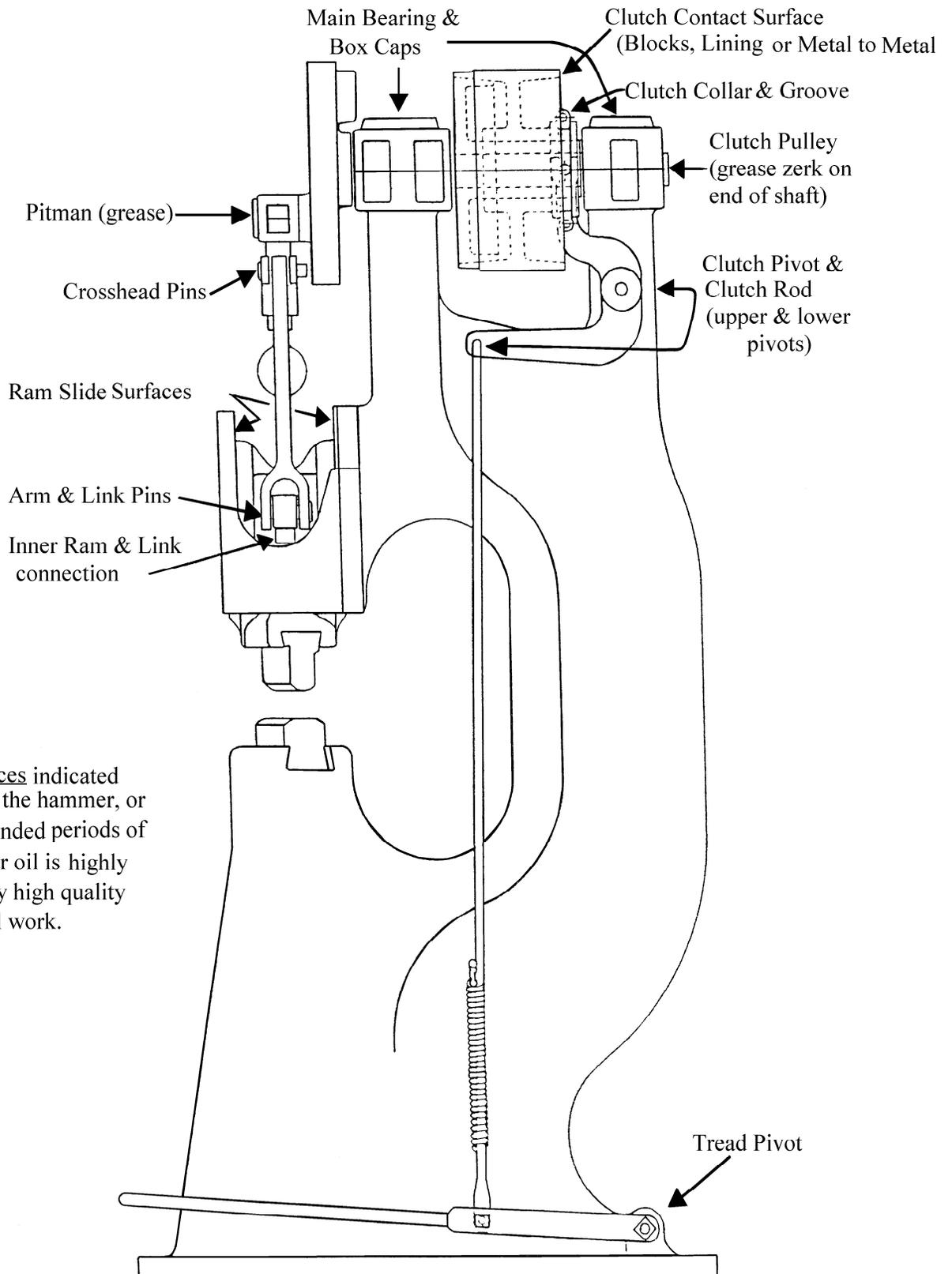
Lubricate all surfaces indicated before each use of the hammer, or hourly during extended periods of use. Chain saw bar oil is highly recommended; any high quality chassis grease will work.
