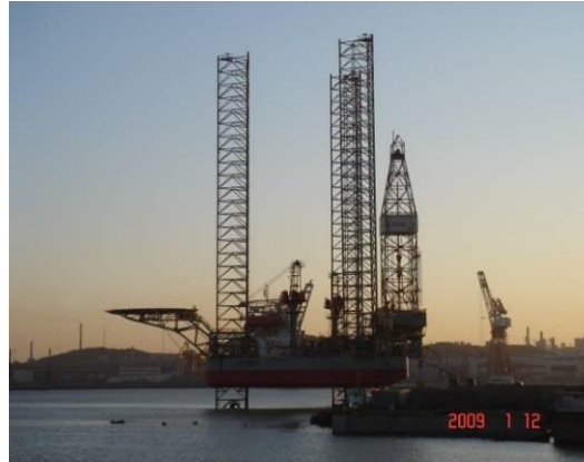
Jack-up drilling platform
