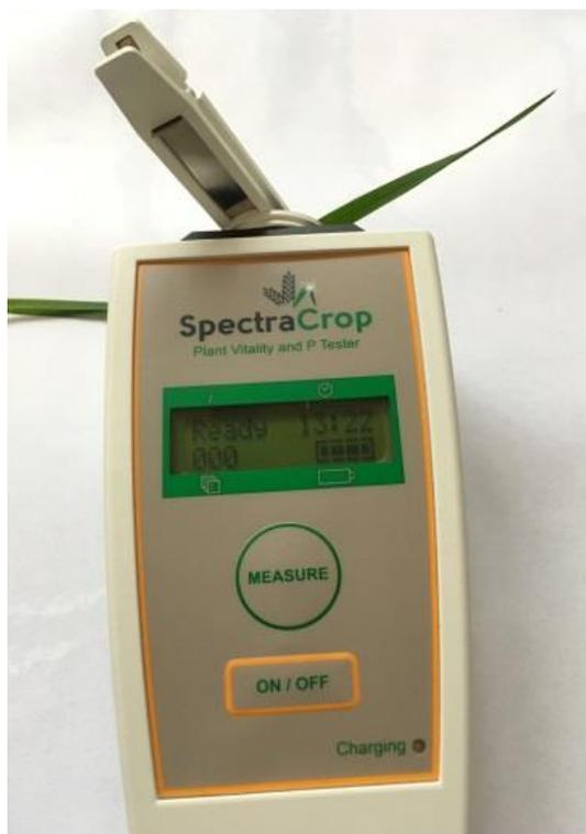
**Figure 5:** The P-tester attached to a leaf clip and ready for measurement. It is critical that the shutter is not opened before a tight fit between the device and the clip is obtained.
