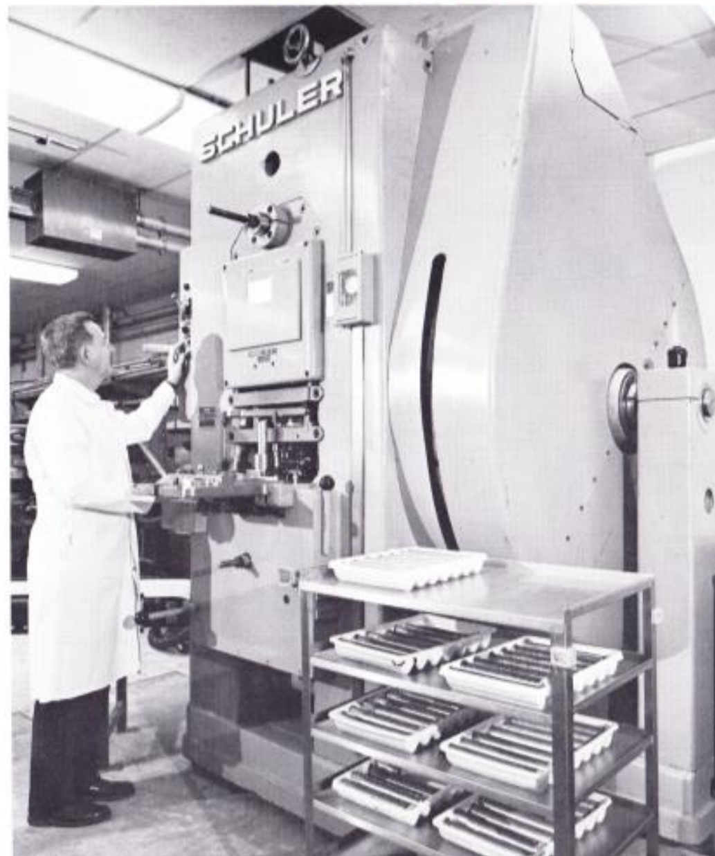
The first of two new automatic-feed coining presses from Germany was installed at The Franklin Mint during the last quarter of 1966. This high-tonnage press is ideal for producing dollar-size coins or tokens at speeds of up to 5,000 per hour—and is the first of its type installed in the United States. An even higher-tonnage version of the same press will be installed in 1967.
