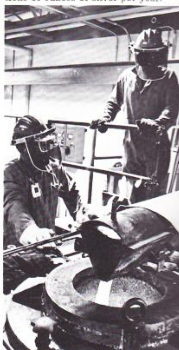
Automated continuous silver casting ment, the first of its type in any mint. The Franklin Mint to melt, cast and millions of ounces of silver per year.
