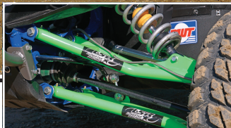
The LSR MTS long-travel suspension utilizes the stock-length shocks. Granlund modifies his own shocks to handle the extra leverage of the longer A-arms. The total width is 71 inches compared to 64 inches stock.
