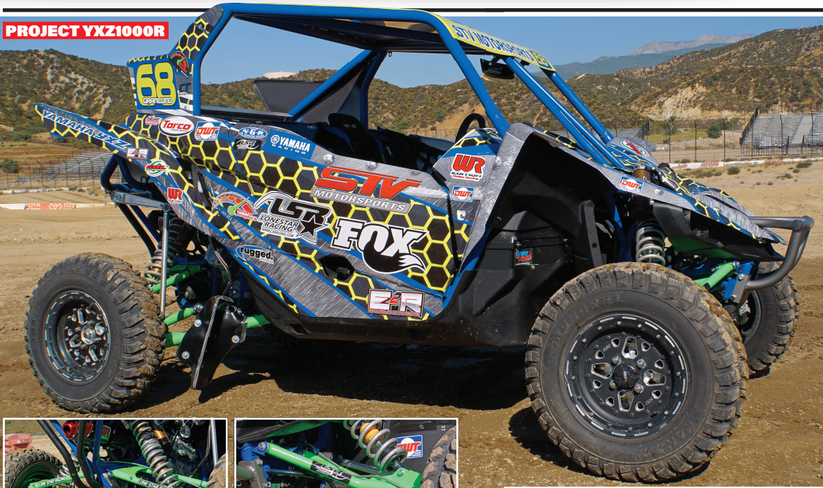
The Weller Racing dual exhaust creates a superbike-esque tone. The Fox shocks are Kashima-coated to help reduce heat and add more performance. The LSR A-arms in the rear complement the front arms perfectly.
