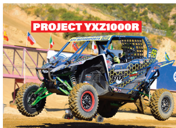
As you can see, the seat position and the lowered cage made for a much lower center of gravity. This helps tremendously with the handling of the car.
