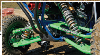
The Weller Racing dual exhaust creates a superbike-esque tone. The Fox shocks are Kashima-coated to help reduce heat and add more performance. The LSR A-arms in the rear complement the front arms perfectly.
