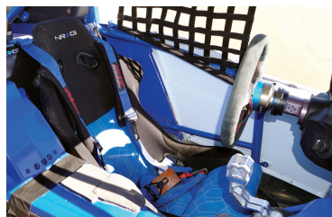
Since Nic Granlund is well over 6 feet tall, he needed more room. His NRG seat sits low and the sides are bolstered. To accommodate him sitting farther back, Hess Motorsports makes the longer steering quickener and mates it with a NRG quick-release steering wheel.
