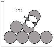
Smooth contact creates less interference, less metal loss and wire deformation.
