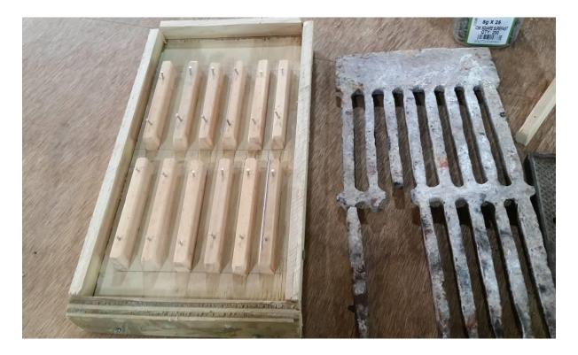
I left the nails sticking up because the bits of wood are tapered the other way and the mould has to come apart, the nails will probably have to be pulled out.
