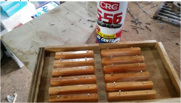
The mortar is a bit dry, and doesn't flow very well due to the fibres mixed in it
