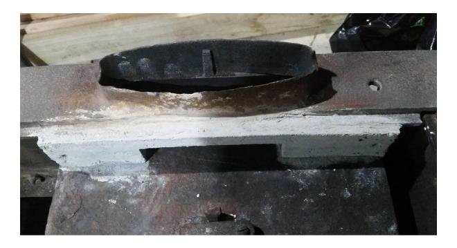
When the top plates go back on, they will need to be cemented in with a suitable fire cement and hopefully we can come up with a suitable release agent. They may need to be re-cemented from time to time but hopefully will last at least another winter. The oven is weak and will eventually have to be replaced with steel (which can be done) but I think the shot is for Marcus to keep his eyes open from now on for a replacement stove.
