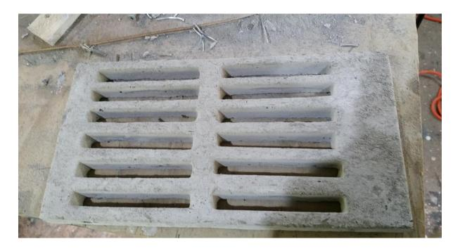
The world's first home-made basalt-fibre-reinforced-cement woodstove grate.
