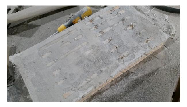
The nails were extracted with a pair of end-cutters and the mould dismantled easily. The casting needed a little fettling, just like an iron casting.
