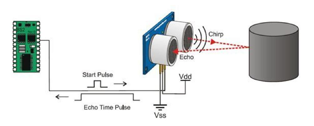
This data is then used to calculate which sensor the user's hand is closest to, and how far away it is. This information determines which button was pressed.
