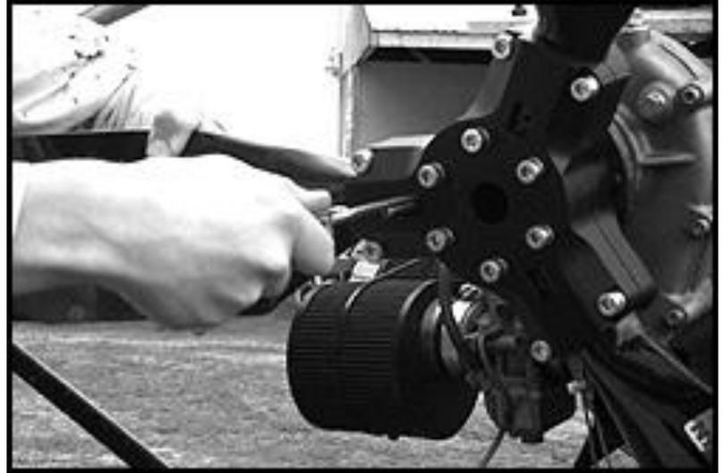
*Figure 10: To use our Speed Set window & pin, place the feeler gauges in the gap between the pin and the window's edge. As long as you are consistent, you can use either side of the pin to set the feelers. Turn the blade firmly, consistently to adjust the pitch to the feelers.*
