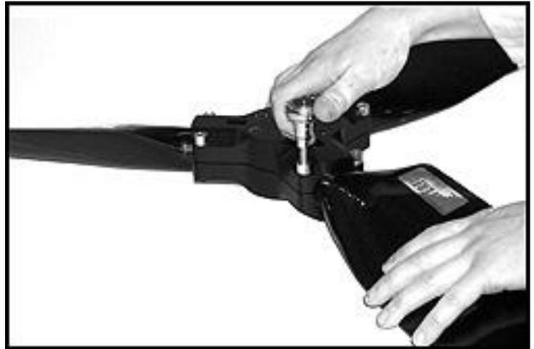
*Figure 4: Insert the bolts evenly, but do NOT torque.*
