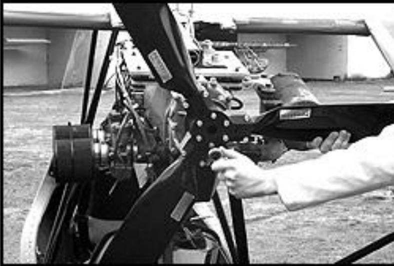
*Figure 6: Lightly snug the center bolts (mounting plate bolts)
