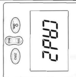
4) Turn the box 90 degrees clockwise; press the ZERO button-the screen will read CA2, make sure the box has no movement until the "2" flash.
