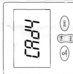
6) Turn the box another 90 degrees clockwise; press the ZERO button-the screen will read CA4, make sure the box has no movement until the "4" flash.
