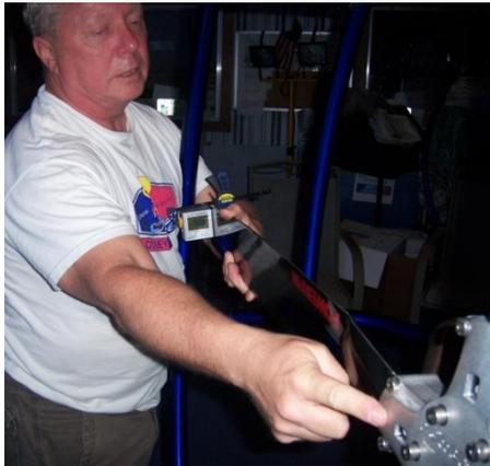
**Pull outward on the blade (from the blade's root toward the blade's tip) BEFORE setting the pitch** to ensure that the blade's shoulder is firmly seated against the inside collar of the Powerfin hub.
