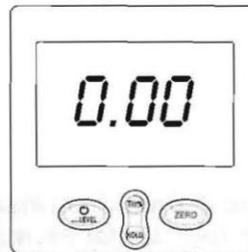
2) Press and hold  $\odot$  and ZERO buttons for 5 seconds until the screen displays CA1.
