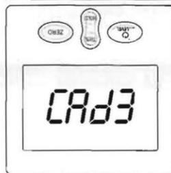
5) Turn the box for another 90 degrees clockwise; press the ZERO button-the screen will read CA3, make sure the box has no movement until the "3" flash.
