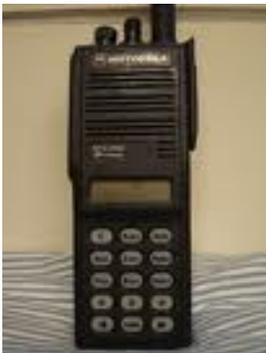
The MTS-2000 handheld radio, used by several City departments, is no longer supported, according to Motorola. As a result, Motorola is no longer accepting orders for the repair of this model.
