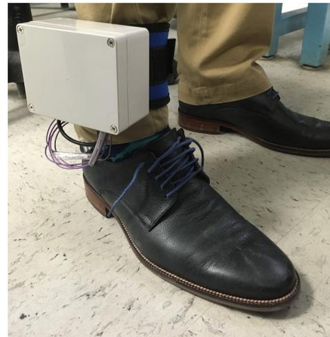
Figure 4: Implemented ankle housing and insole in use
