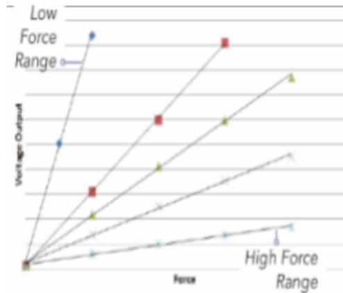
Fig. 3. Voltage output of the drive circuit as a function of the applied force. Note that the various plots are all depending on the chosen value of the fixed resistance value from the negative op amp terminal to the output, and can be used to select the sensitivity of the sensors.
