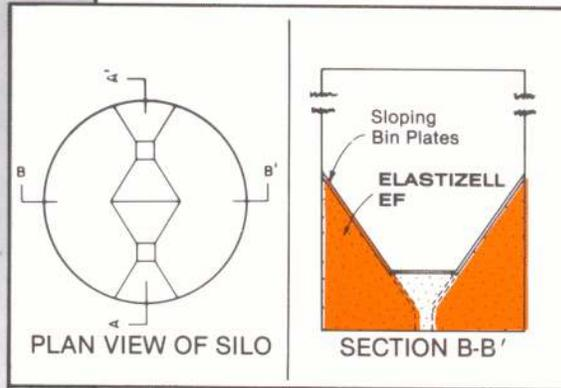
**ELASTIZELL EF** fills the void behind the sloping discharge hopper plates (supported by bar joists) and the slipformed silo wall.
