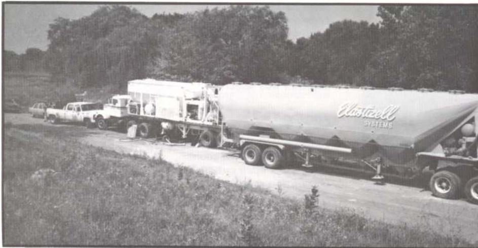
Specialized batching, mixing and placing equipment is required for the proper installation of **ELASTIZELL EF** for pipeline fill voids.
