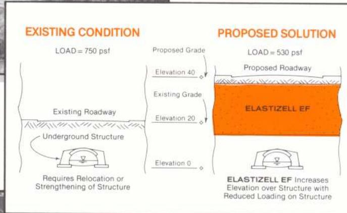
**Elastizell EF Reduces Loading Over an Underground Culvert Structure Unable to Support Additional Loads.**
