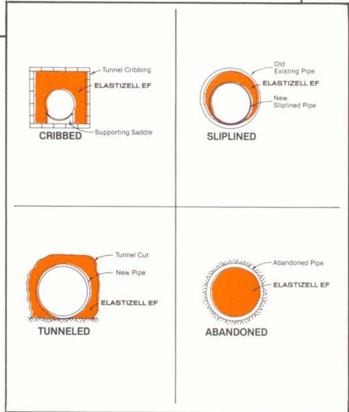
High flowability of **ELASTIZELL EF** completely fills voids from various types of pipe line construction. **ELASTIZELL EF** will not overload poor soils and is much stronger than other backfill materials.
