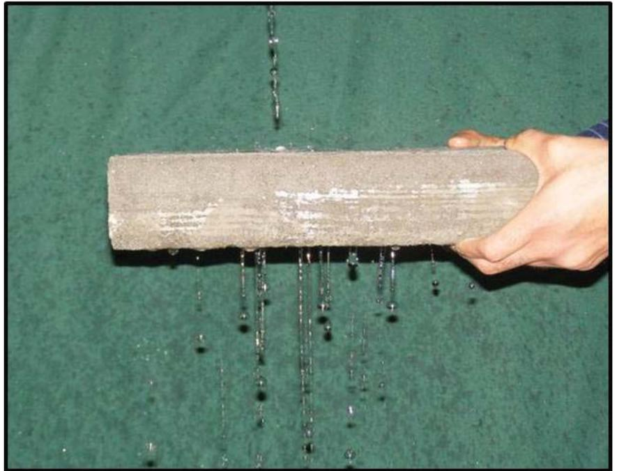
The use of lightweight cellular concrete continues to increase worldwide. New products from Aerix Industries™ are helping to drive this powerful trend, including the introduction of AQUAERiX™, a patented synthetic foaming agent for production of pervious cellular lightweight concrete. (Patent No. US 8,172,937 B2)
