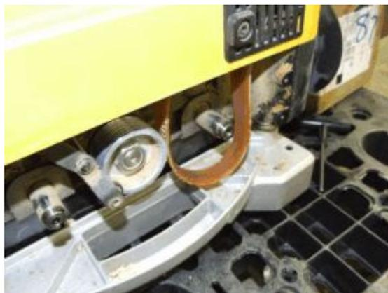
11. Remove the nut from the end of the head.
