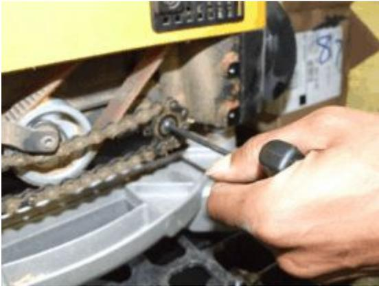
9. Remove the chain and sprockets together.
