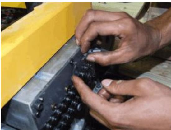
17. Remove the chain and sprockets together.
