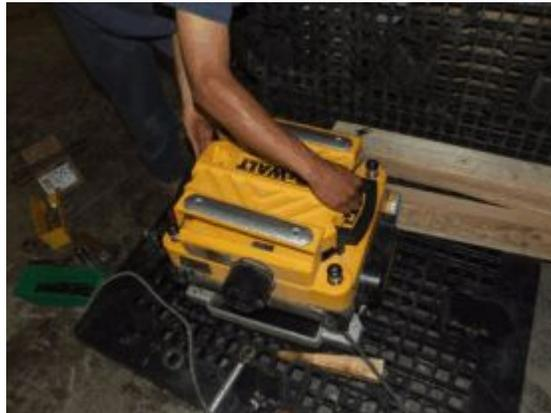
2. Remove the 3 red thumb screws from the inside of the top, then remove the inside dust cover. Doing this will expose the cutterhead.
