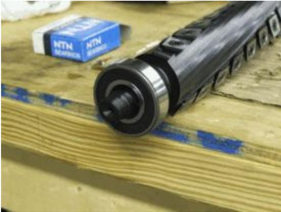
25. Carefully slide the new head through the bearing housing. Be careful of alignment so as not to bind the carbide knives and chip or break them. You can wrap the new cutterhead with blue painter's tape to help protect the carbide knives.
