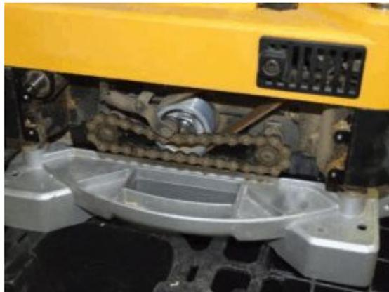
7. Unhook the tension spring and remove the idler arm, being careful not to strip the Phillips head screw which is held in place with blue thread lock.
