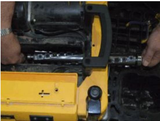
26. Carefully tap the head into position making sure the bearings are fully seated in the housings.
