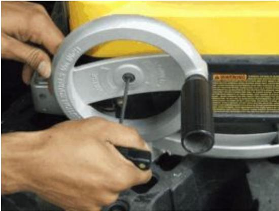
6. Remove the 4 screws and cover. This will expose the feed chain and pulley.
