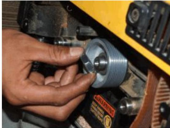
12. Slide the pulley off taking care not to lose the key, and remove the bushing from the shaft.
