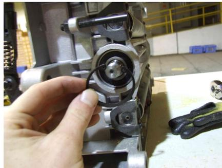
13. From the side opposite of the pulley, tap the head out using a block of hardwood.
