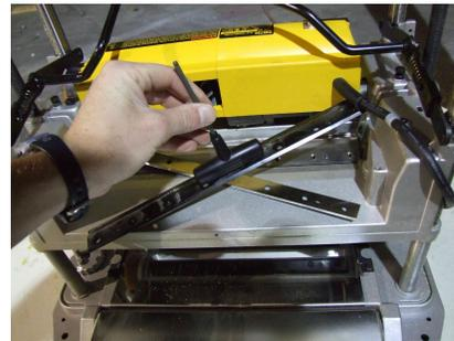
4. Remove the rotate lock by removing the spring first and then the lock itself.
