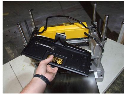
3. Remove the 3 blades from the cutter head by taking off the screws and clamp bar.
