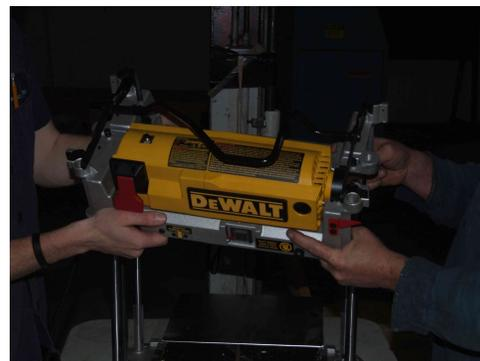
7. Remove the gear cover by removing the two screws. One on each side.
