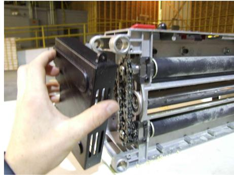
8. Remove all three snap rings on the gears. Pull off the gears. (be sure to not lose the spacer on the front gear)
