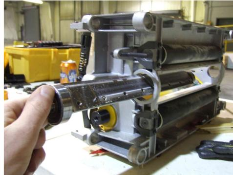
14. To install the SHELIX ®. Carefully maneuver the head into the bearing housing. Watch the alignment so you do not damage the carbide tips.
