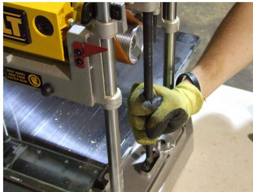
6. Once the assembly is off the threads carefully maneuver the assembly off the posts.
