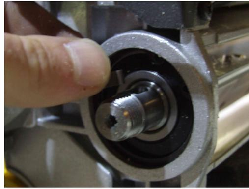
12. Remove the snap ring holding the bearing in place.
