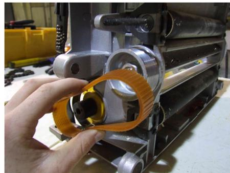
10. Remove the nut from the end of the head. A piece of wood will help hold the head in place.
