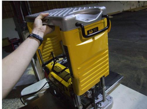
2. Remove the chip breaker by removing the two screws on each side with the wrench provided.
