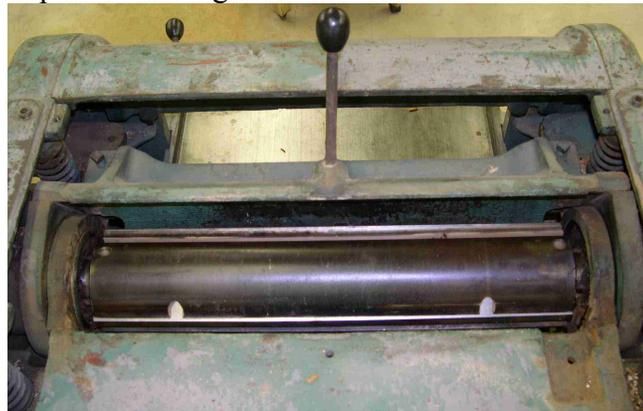
9. To avoid serious cuts and binding of the planer knives when extracting the cutter head through the chip breaker and pressure bar hangers, remove the old knives, shims, and lifters from the cutter head.
