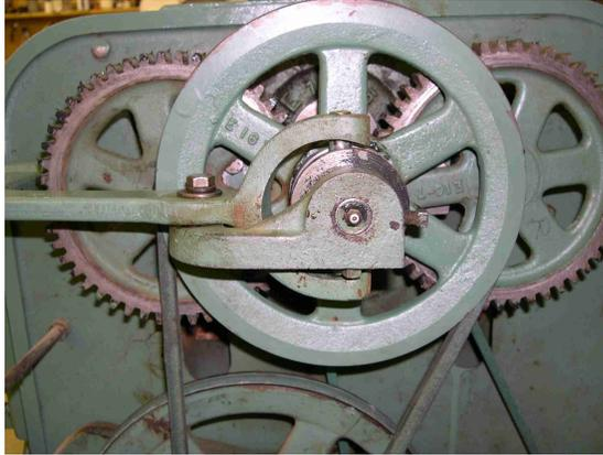
13. Remove the large gears on the in-feed and out-feed rollers.
