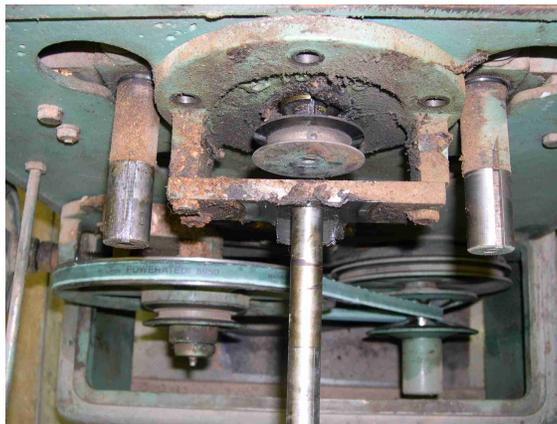
15. Remove the grease fitting on the right bearing housing assembly BEFORE pulling the housing. Pull the right bearing housing assembly.
