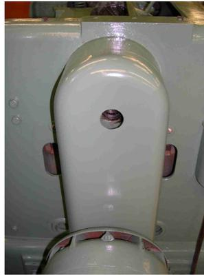
5. Remove the large guard on the right of the planer that covers all drive gears, clutch, etc., and belts.
