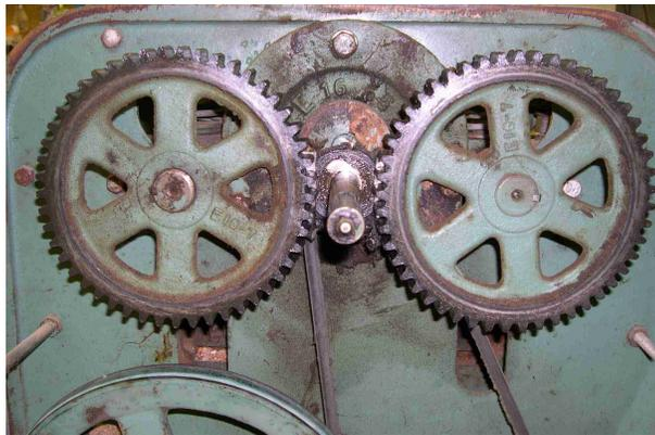
14. Remove the mounting bracket assembly on the right side to allow direct access to the cutter head shaft on the right and easier use of the bearing puller. Remove the four bolts in the bearing housing assembly.
