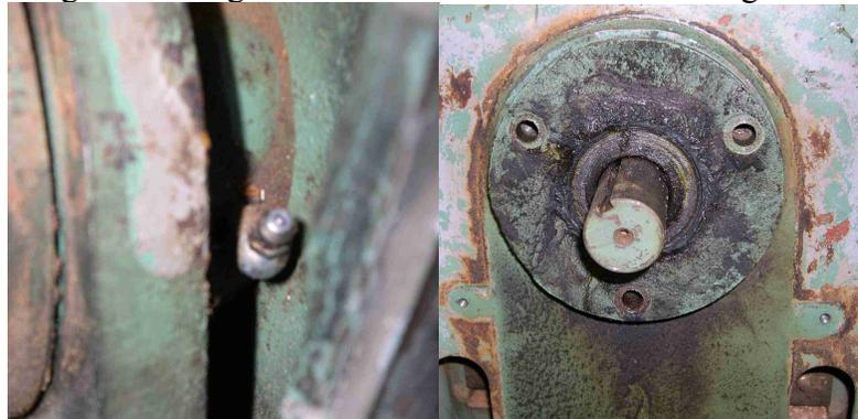
11. Use a bearing puller to remove the left bearing housing assembly. (Most likely the bearing will remain on the cutter head.)
