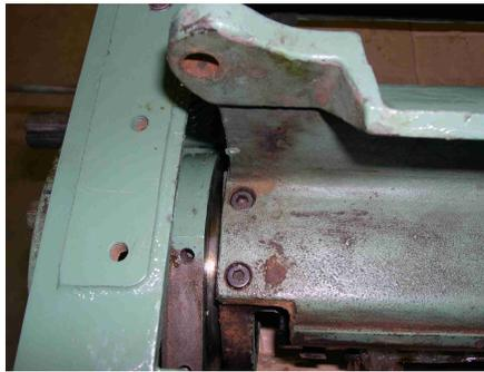
18. Remove the Allen head bolts and the pressure bar.
