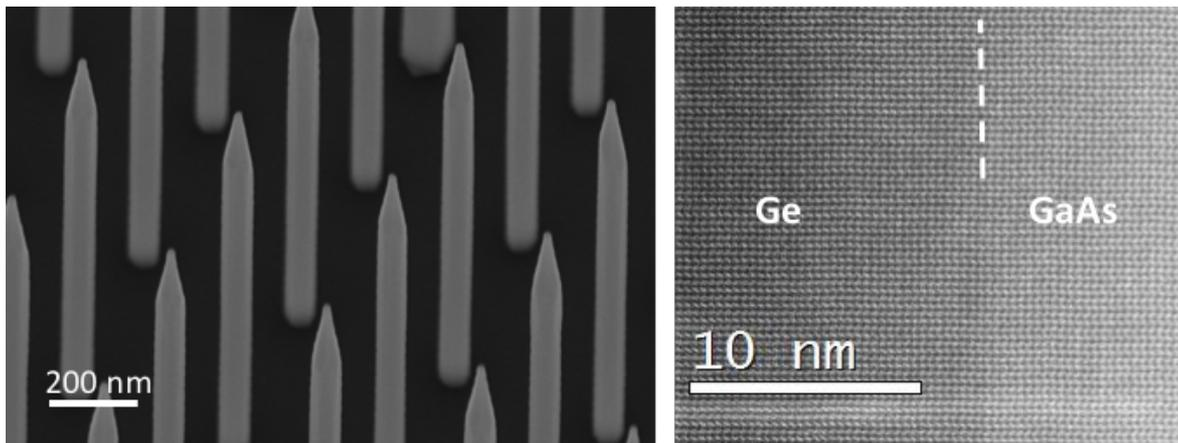
Figure 5. SEM image of WZ GaAs wires. E-beam lithography has been used to define the position of the Au catalysts in a SiN capping layer on a GaAs(111)B substrate. HR STEM image of the interface between the WZ GaAs core and the hexagonal Ge shell. From this image the epitaxial relation is clearly visible.
