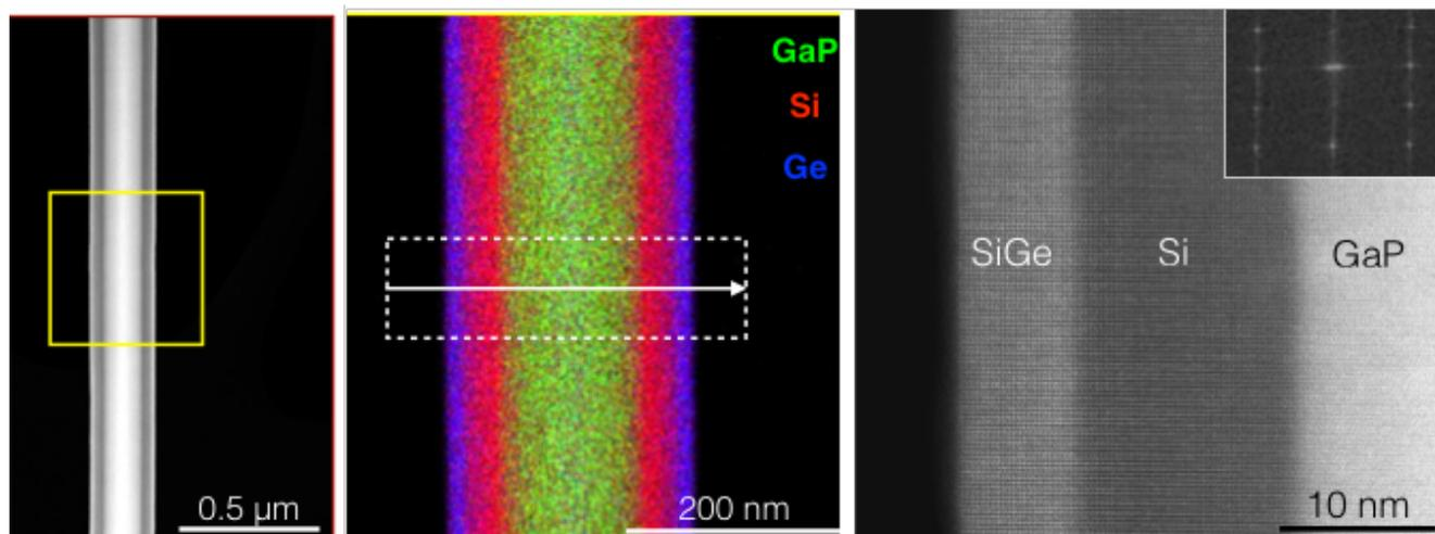
Figure 1. Overview TEM image of a hexagonal GaP/Si/SiGe core/shell/shell wire show the uniformity and defect-free nature of the wire. Elemental map of the wire showing the composition of the structure. HRTEM image of the wire demonstrating the hexagonal crystal structure. We note that a thin wire with a thin shell has been used for imaging, since it is very difficult (impossible) to obtain high resolution images from thicker samples.
