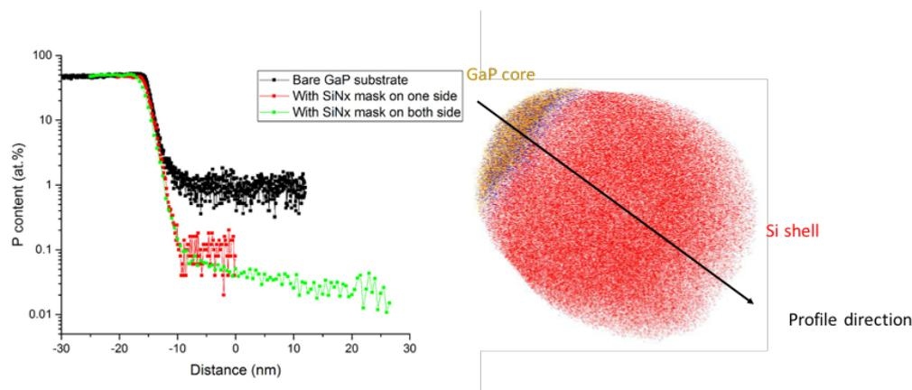
Figure 2. Atom Probe Tomography (APT) line scan of a hexagonal GaP/Si core/shell nanowire. Au and Ga are below the detection limit (1 ppm) of the APT. The P concentration in the Si shell is the highest (1%) when an uncapped GaP substrate is used and the P concentration decreases with the level of capping the GaP substrate.
