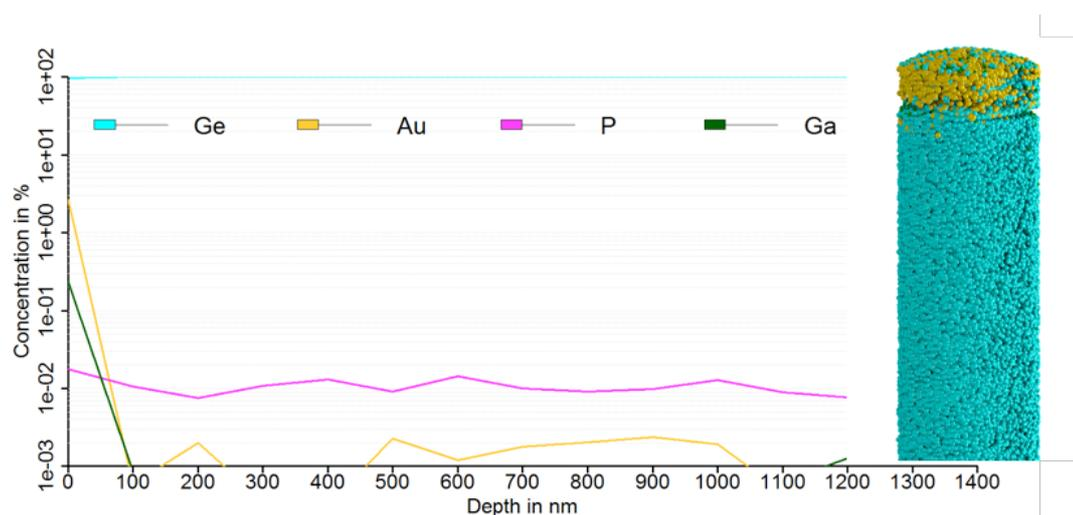
Figure 4. APT line scan of a hexagonal Ge branch grown from a WZ GaP stem wire. The reconstructed image shows Au atoms at the top of the wire (catalyst particle), and Ge atoms in the wire.
