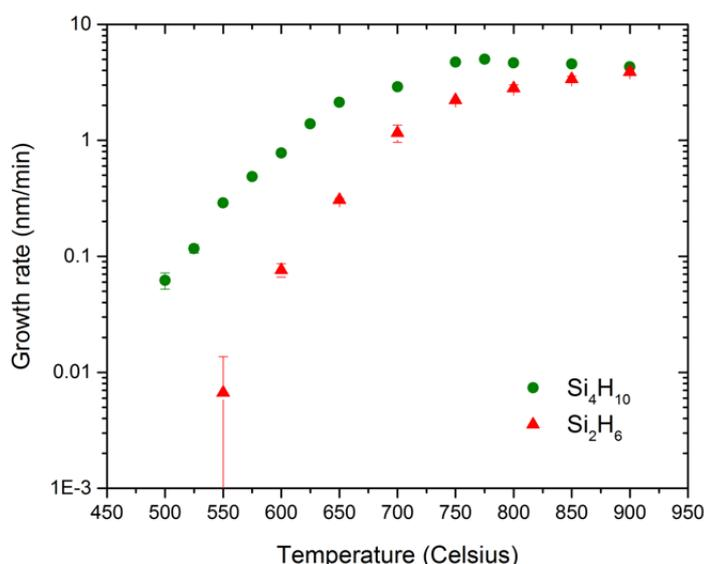
Figure 3. Growth of the hexagonal Si shell on WZ GaP core wires for two different precursors. Below 700 °C the growth rate with tetrasilane is 3-10 higher than with disilane due to the lower cracking temperature. We note that the real substrate temperature is 80-100 °C lower than the thermocouple set point temperature (T on x-axis) due to the thermal contact.
