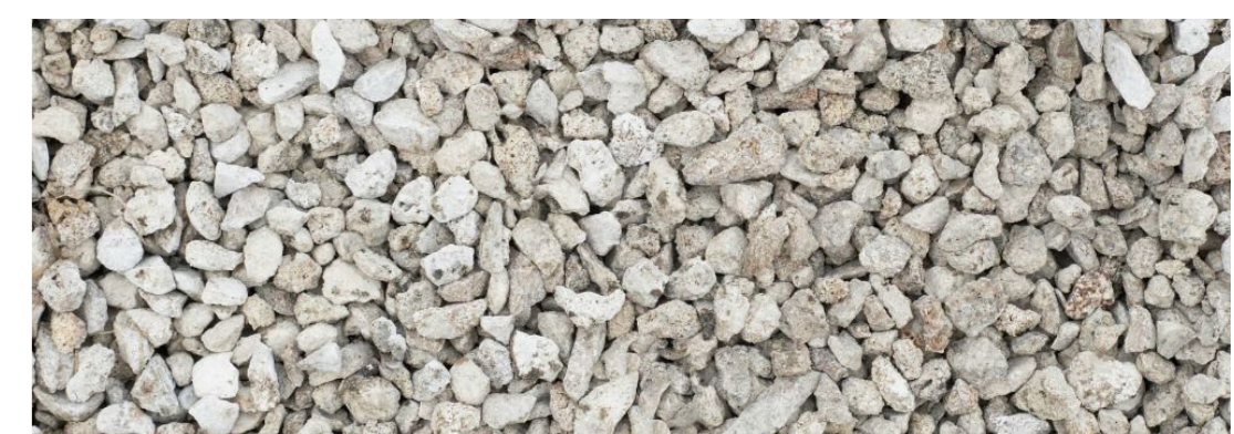
Reclaimed and crushed concrete
