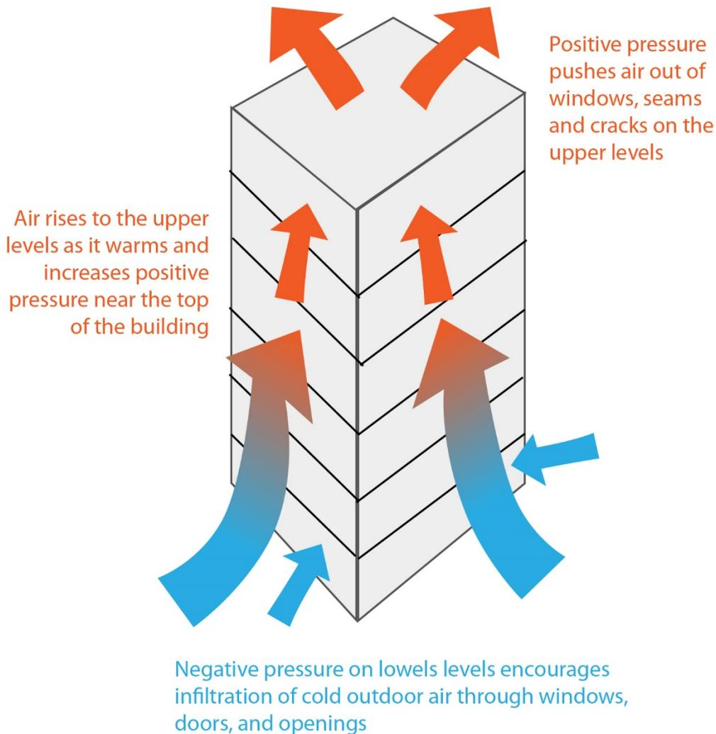
I was referred to a building because they were having extremely high energy bills. The first thing I noticed was that the doors were blowing open. Common sense; if you're blowing your conditioned air out, warm outside air is coming in via the HVAC system.
