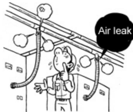
The pneumatic dampers were not opening the cooling enough to allow the air to condition this end of the building. So, by fixing the simple air leak I was able to reduce energy consumption significantly and save the facility \$180,000 in repairs. Again, with technology today there is a simple cost justified diagnostic solution.
