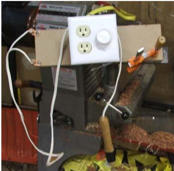
And here's a close up of the working end of Steve's DIY "pen". Note that the bare copper wires between the plastic covered terminals on the end of the handle and the bare terminals connection to the nichrome wire on the pen tip acts as heat sinks, reducing the heat from the hot pen tip before it gets to the plastic insulated terminals.
