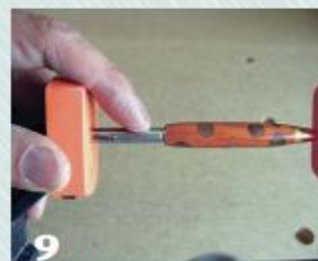
9 Press fit the pen parts together.
