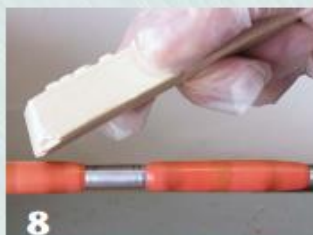
8 Apply and buff coats of wax on the pen barrels.
