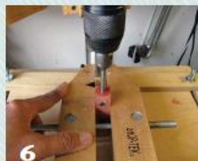
6 Square the ends of the pen barrels to the brass tubes.
