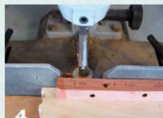
4 Use a mortising machine or drill press attachment to cut the square holes. You can also cut them by hand with a chisel and mallet after drilling a smaller hole within the square.
