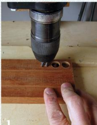
Chuck a 1/4" plug cutter in the drill press to make plugs of a contrasting wood.
