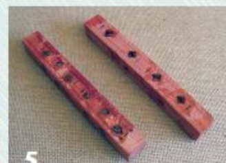
5 Glue the plugs and square pieces into the drilled voids.
