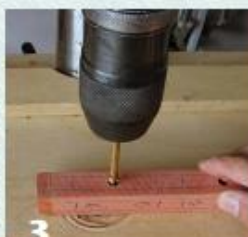
3 Drill all the 1/4" holes in the blanks using a drill press.
