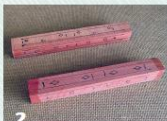
2 Use a dark pen to lay out your design and boundary lines based on the finished diameter of the pen.
