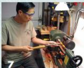
7 Turn the pen barrels to the desired profile and size.
