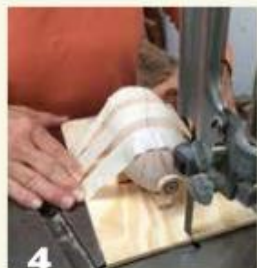
The author's pod cut in half on a curved line. The tenons at each end can be cut off after the pod is split.
