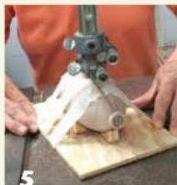
The author's pod cut in half on a curved line. The tenons at each end can be cut off after the pod is split.
