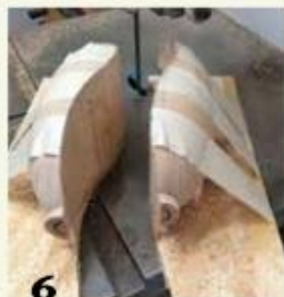
The author's pod cut in half on a curved line. The tenons at each end can be cut off after the pod is split.
