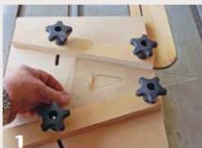
1 Use a 30/60/90 triangle to set the fences on your table saw sled to the desired angle.
