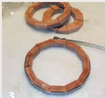
3 Glue the segments into rings, using a band clamp to apply even pressure.
