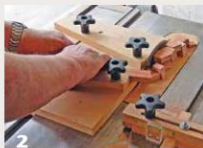
2 Cut the individual segments. The length of all segments is made identical with the use of an adjustable stop (bottom right of photo).
