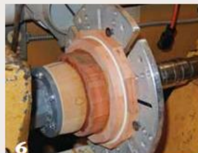
Three methods of centering a ring when gluing it to the previous layer. Use a ruler or your fingers as a gauge, or mount the ring in large chuck jaws mounted on your tailstock.
