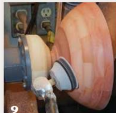
9 Sand your segmented bowl, apply finish, and part or cut it off the lathe.
