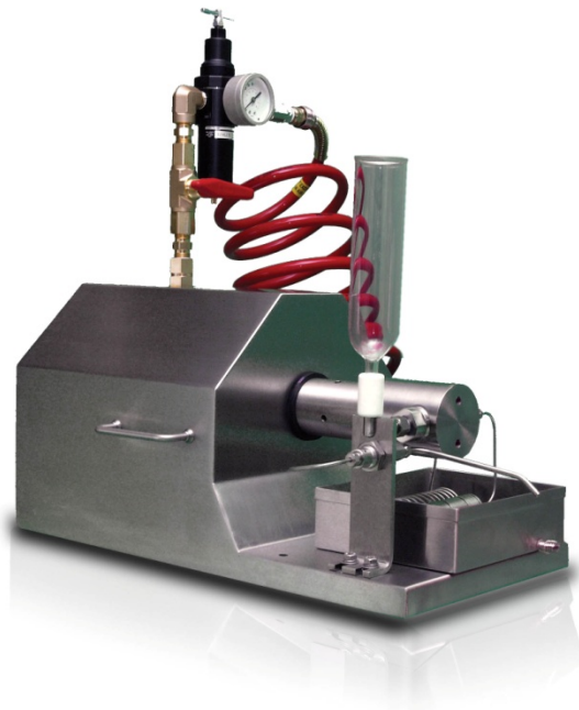
Fig. 3 Model M110L Microfluidizer processor (Microfluidics, Newton, MA, USA) equipped with a ceramic interaction chamber.
