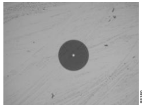
Figure 12 a damaged Connector with a 1.25 mm ferrule that has been over chamfered. The connector must be replaced.
