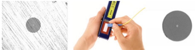
Figure 7 The contaminated endface (left) shown in this fiberscopic image is cleaned with a cassette type hand cleaner(center) and, when re-inspected, is found to be clean (right). (Photo courtesy of Photonics Spectra June 2004) (2)
