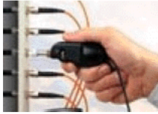
Figure 5 Handheld probe inserted into a bulkhead connection (Photo courtesy of Fluke Network)
