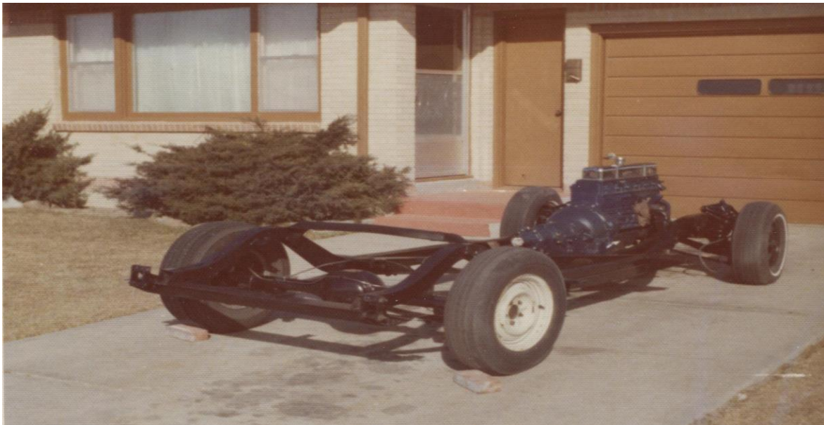
Frame and engine completed
